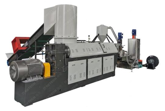
Plastic PE PP film recycling pelletizing machine is used to processing and granulating washed LDPE film,LLDPE film,PP woven bag,HDPE film bag,etc. With new advanced technology from Europe and continues feedback comments from customers,RETECH got rich experience on design&manufacturing PP PE film pelletizing lines.
